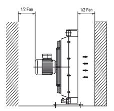
The cooler is normally installed in the return line of the oil circuit. It must be protected against shock loads and mechanical vibrations and not subjected to imposed strains or vibrations. This is normally achieved by connecting the cooler to the equipment using hose lines. Do not expose the heat exchanger to pressure shocks, pulsations or sudden changes in flow rate. This can lead to irreversible damage of the cooling element.
