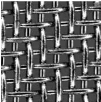
Wire mesh • 10/25/40/60/100 \mu\text{m} • Regeneratable (e.g. in an ultrasound bath)
